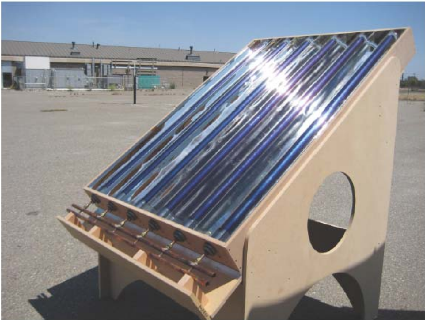
XCPC Solar Thermal Collector at UC Merced Solar Testing Facility
